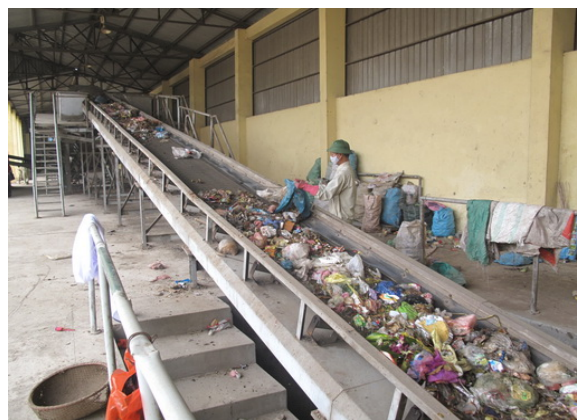
Photo 11: Chain of waste separation in Kieu Ky composting plant(Gia Lam District)
